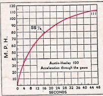
Specifications at a glance: Four cylinder, overhead valve engine; displacement—2660 cc; 90 bhp at 4000 rpm; wheel base—90 inches; curb weight 2150 lbs.; distribution 49%/51%; three forward speeds plus overdrive (synchromesh); steering 2½ turns lock to lock; brake area 145 square inches; average fuel consumption, 25 mpg.
