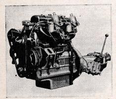
The Austin-Healey's competition-tested engine develops its maximum torque at a modest 2,000 rpm for top acceleration through the gears. And not only is the engine reliable but it's easy to maintain too, with parts (including a modification kit) quickly available from 14 Austin distributors and 350 dealers.
