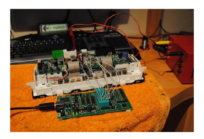
Ok, going carefully with where goes every wire on the willem, we setup our software and read the eeprom content. I selected in my software 93c56B (16 bits) (important set to 16bits), I was able to read it a max speed (called "+2" in my case).
