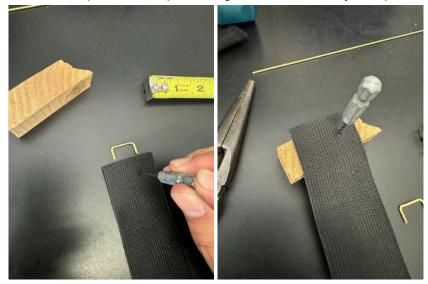
6. Poke the staples through the strap. I preferred to put the folded side of the strap down as seen below.
