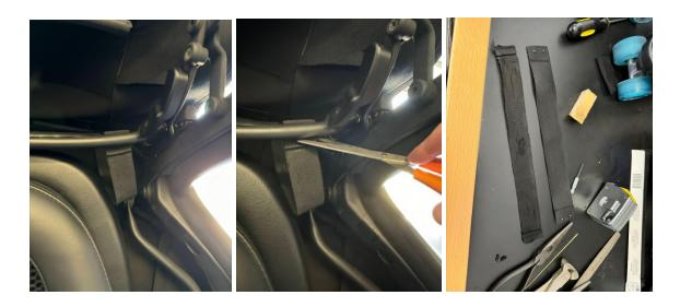
10. Start by wrapping the rear end of the strap on the back bar, then wrap it a full 360 degrees around the bar and insert the staple legs into the center holes in the rivets. Ignore the second strap you see in the picture to the left, I have an AP1 and retrofitted the top with a glass window on it.
