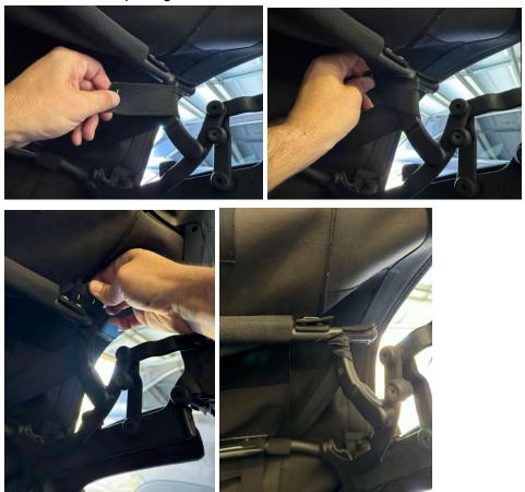
13. Next pull the strap that is wrapped around the side bar and lift it up and over the top bar so it will straighten it all out
