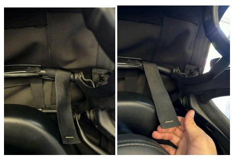
12. Next, pull the front end of the strap around the post like this, then wrap it up to the top and insert the staple legs in the rivet center holes.
