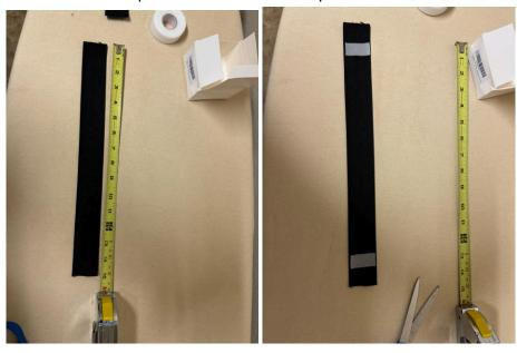
3. Flip the end over and overlap it approx 1" so the adhesive strip is inside two parts and iron the ends to activate the adhesive. Do the same for both sides and make it so the full length of the strap is 12.5" long. (adjust this length as you see fit for your preference)
